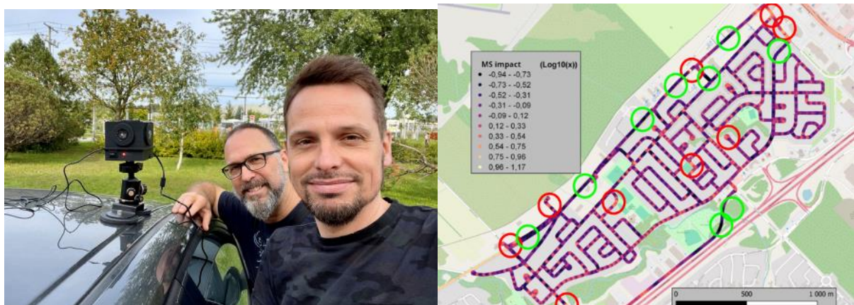
Fig. 1: M. Aubé and S. Poulin installing the LANcube on car roof (left) and an example of melatonin suppression impact map for a Quebec City district (right). Red circles identify high melatonin suppression impact regions while the green circles highlight low impact.
