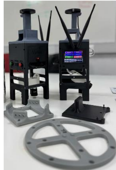
Fig. 1: Vultur device and three mounting accessories for platforms
