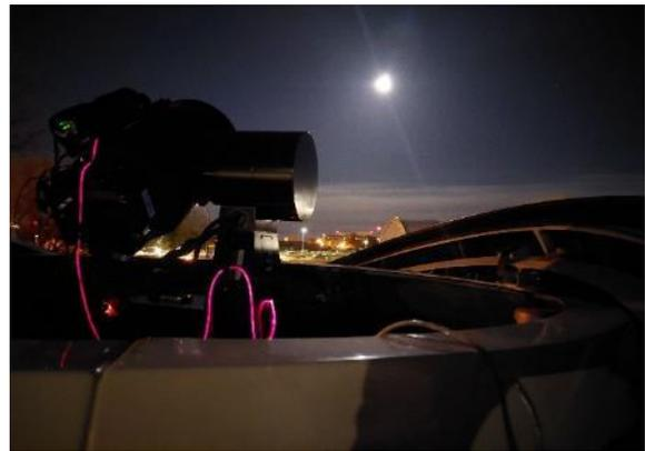
Fig. 1: The optical quantum ground station located at the University of Calgary. This computer controlled 280 mm telescope is one of the primary instruments used to collect data for the analysis of anthropogenic light pollution in the Calgary metropolitan area. Photo: Mathew Yastremski
