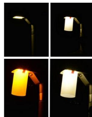
Fig. 1: Top row: Street lights without (left) and with diffuser (right). Bottom row: amber LED color temperature and neutral-white color temperature. Photos: Martin K. Obrist, WSL
