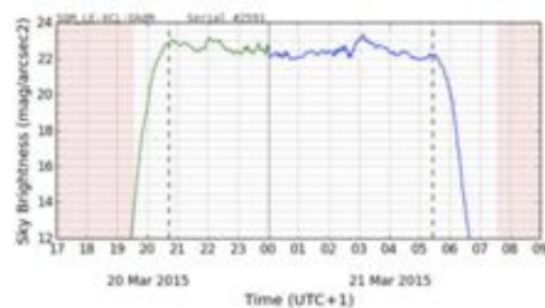
Fig 2: NSB evolution in a cloudy night. There are continuous and not smooth changes in the evolution of NSB.
