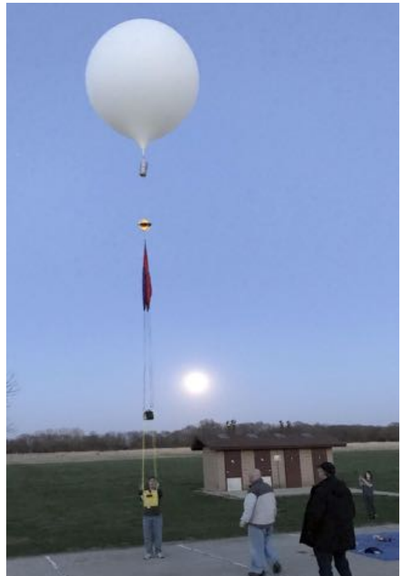
Fig. 2: Launch of a NITELITE test mission showing the configuration of the flight elements.
