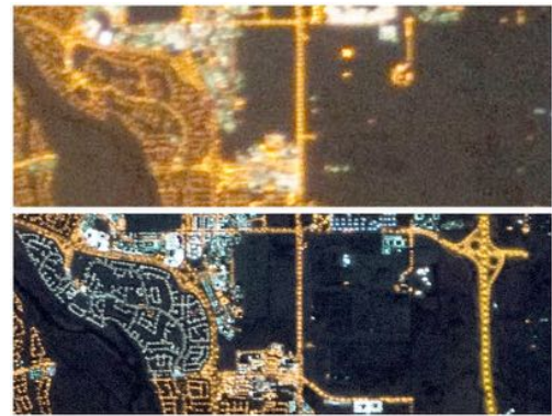
Fig 2: Lighting change in a 22km 2 portion of Calgary, Alberta, Canada, from 2012-2015. At left, a neighborhood changed to white LED, at right, a ring road is newly lit with HPS lamps. Images ISS026-E-12438 and ISS045-E-155029 courtesy of the Earth Science and Remote Sensing Unit, NASA Johnson Space Center.
