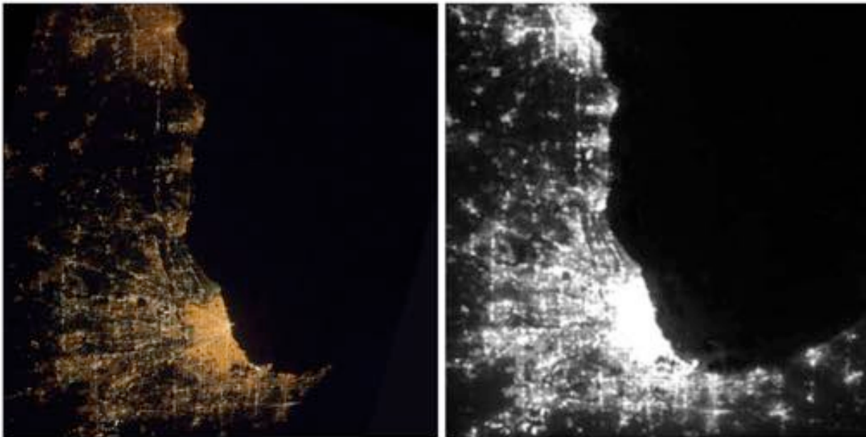
Fig 2: Simulated NITESat (left) and actual VIIRS (right) images of the Chicago region. NITESat will provide a 3-fold increase in resolution over VIIRS as well as invaluable broad-band color data. NITESat simulation is a down-sampled image from the ISS. Image credits: Earth Science and Remote Sensing Unit, NASA Johnson Space Center and VIIRS Image and Data by NOAA's National Geophysical Data
