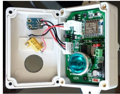
Fig 1: Optics and electronics of the STARS4ALL TESS-V1 photometer inside its weatherproof enclosure.
