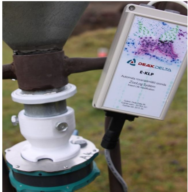
Bottom of the Jermy light trap, ZooLog sensor ring and data collector have been connected .
