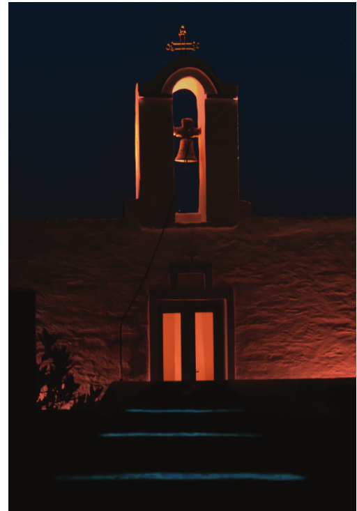
Fig. 1: Rehtink the Night – example of techniques : Chapel of the Archangel Michael with candle-flame graduation and linear applications of phosphorescence to the paving serve as “guide-lights”. CC-BY
