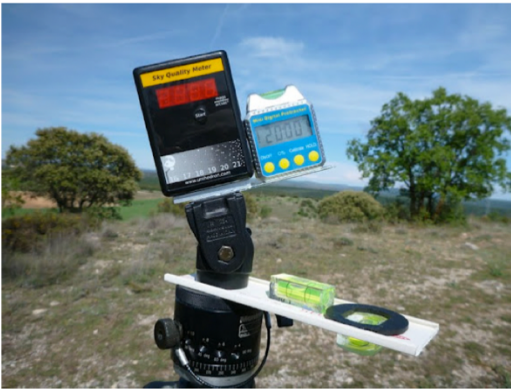
Figure 1. The SQM photometer fitted to a graduated tripod was the original instrumentation used to obtain the data to build the NixNox all-sky brightness maps.
